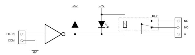
Electrical circuit diagram for a single relay channel.
