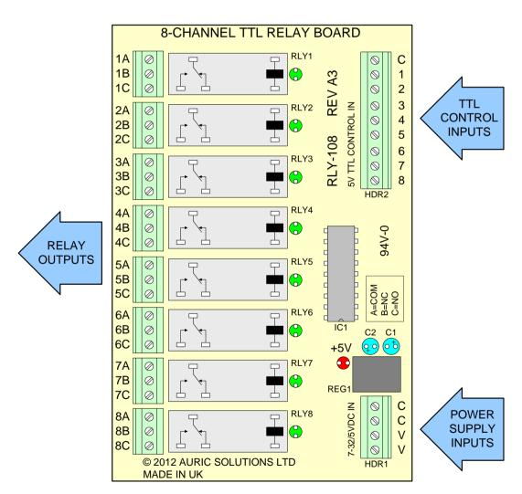
Component layout on the RLY-108 relay board.
